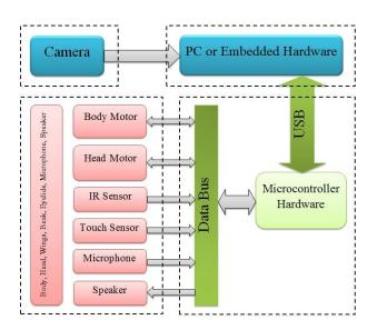
Fig. 2. The RoboParrot schematics
