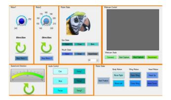
Fig. 8. The RoboParrot User Interface. The top-left boxes are the control for the body and head motors. The top-middle box, with the parrot head, shows the states of the robot's eye and beak. The top-right box is the camera view. The bottom-left gauge shows the sounds level. The bottom-middle box are different songs that can be played for a child. The bottom-right box are specific controls that the operator can select such as moving left or right and opening-closing wings
