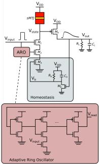
Fig. 1. The S4N circuit developed herein.
