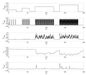
Fig. 2. The operational waveforms of the S4N circuit.
